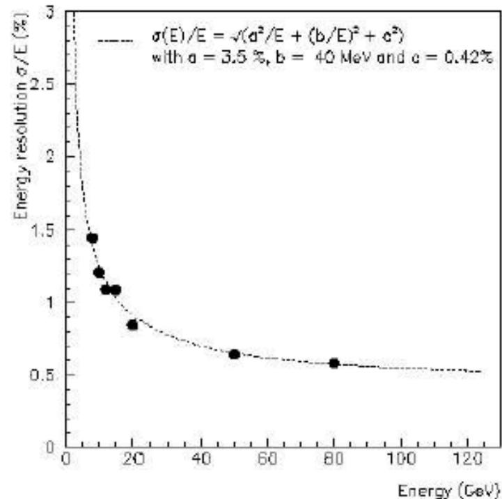
FIG. 3 Fractional electron energy resolution as a function of energy measured with a prototype of the NA48 liquid krypton electromagnetic calorimeter (NA48 Collaboration, 1995). The full line is a fit to the experimental points with the form and the parameters indicated in the figure.
