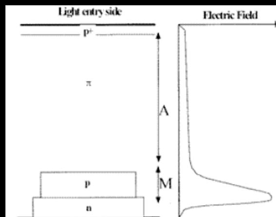
Figure 1: Reach-through APD Structure (Not to Scale)
