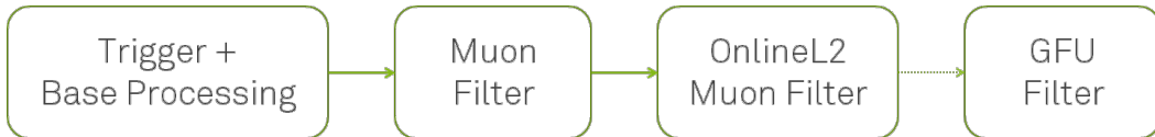
Figure 2.2: An example processing chain for the gamma-ray follow-up (GFU) filter is shown. The Muon Online L2 Filter is the basis for many different follow-up programs.
