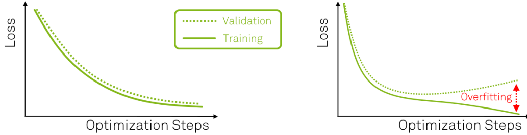
Figure 6.1: Overfitting of the training data can be monitored by evaluating the loss curves for the training and validation set. On the left, a typical loss curve is shown in the case of no overfitting, whereas the case for overfitting is shown on the right.
