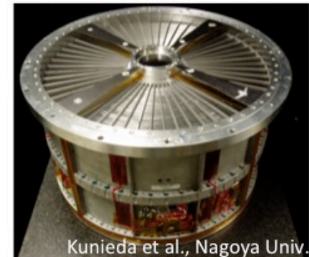
255 shell Al mirror with 50 cm 2 area at 30 keV (Pt/C coating).
