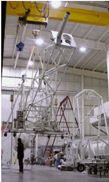
InFOCUS gondola with 8m optical bench (Tueller et al., NASA GSFC)
