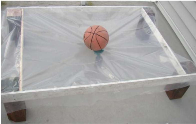
*Several views of a simple rooftop collector. The basketball creates a belly in the plastic, keeping it from flapping in the wind. Below the ball is a hole, so that rainwater can wash the plastic into the blue funnel, held up by a can with gravel in it. Runoff passing through the funnel runs near a strong magnet (not visible) on the outside of the funnel. Iron-rich particles are captured on the inside of the funnel and can be removed for study.*
