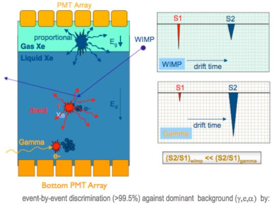
· Simultaneous Detection of scintillation (S1) and ionization (S2)
