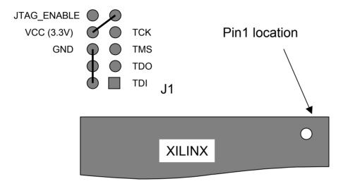
Connect VCC only when the flasher board is not plugged into the DOM main board. Connect JTAG\_ENABLE to VCC in order to enable JTAG programming.
